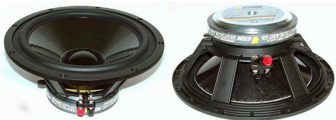
The midwoofer: The original [Scanspeak 18W8545](#) had proven it's qualities with a low resonance frequency of 28Hz, a large long throw 42x19 millimeter voice-coil and a very large magnet to give a strong driving force. The cone is made of carbon fibre filled
